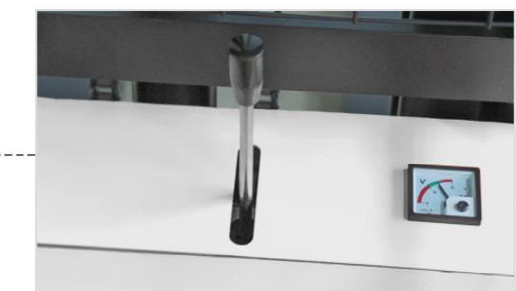
Use handle to control fork height electrically
