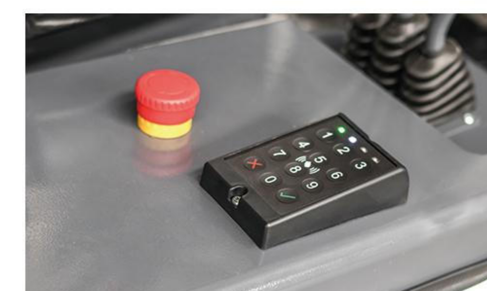
Emergency switch + Pin-code lock
